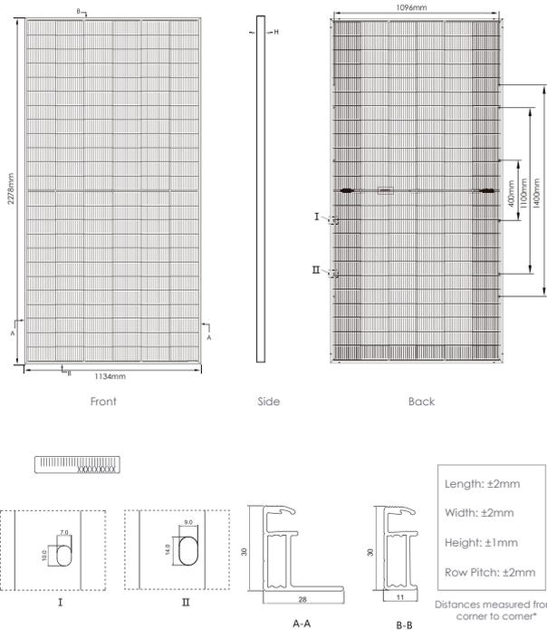
\*For detailed sizes and tolerance specification, please consult detailed module drawing
